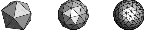
Figure 1: Discrete samplings of the sphere corresponding to order 1, 2 and order 3 of tessellation of an icosahedron, with correspondent |T_1| = 12 , |T_2| = 42 and |T_3| = 162 points.
